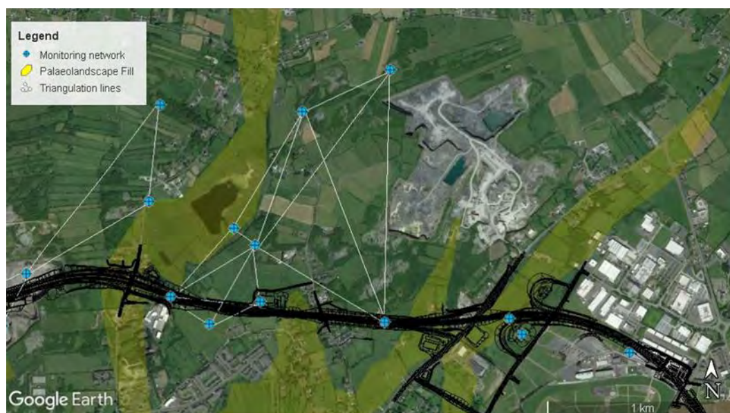
Plate 4 Example of the triangulation net used (June 2016 water levels)
